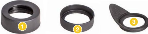
1. The standard eyecup is the large height-adjustable eyecup that also fastens onto the M43 photo-thread of the eyepiece. By rotating it counterclockwise, the height will increase. This eyecup easily unthreads by simply rotating it upwards further than the uppermost stop – this reveals the M43-thread connection. This eyecup is preinstalled when the eyepiece is shipped and the most common eyecup for use with a telescope.
